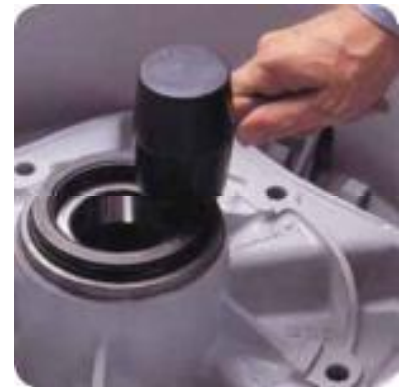
A rubber mallet may be used to tap into place.
