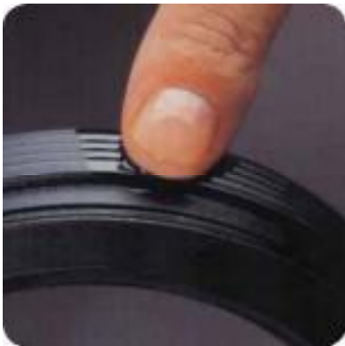
Lightly lubricate the OD and ID with the fluid being retained. Never install dry.
