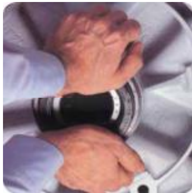
Press the seal into the bore with the palms of your hands. Use even force to avoid cocking the seal and be sure that the seal is evenly seated and bottomed in the bore.
